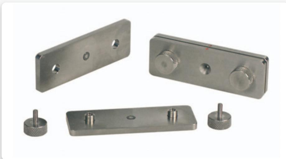
The DC-2 is a unique diamond compression cell comprising of two type IIa diamonds, each metal bonded into a Hastelloy plate.
