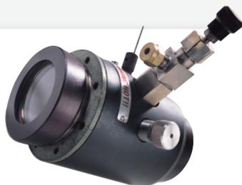
thermocouple port and vacuum valve. Windows are secured using threaded end caps and chemically resistant seals. The cells can be dismantled to allow easy cleaning and window replacement.
